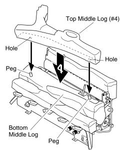
Figure 19 - Installing Top Log (#4)
